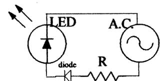
Above; Typical AC circuit using a diode. The "R", or resistor is not necessary for 12-14 or 24-28 volt assemblies when they are used @ rated voltages.
