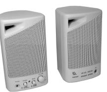
A shielded speaker pair for use with a personal computer system. The built-in audio amplifiers produce up to five watts per channel; and a frequency response from 120 to 20,000Hz. Volume and bass controls are on the front of the speakers, as well as a headphone jack for private listening. The system is powered by an AC adaptor; included. Each unit is a compact 4" wide, 4.5" deep and 6.5" tall.
