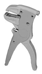
This compact, self-adjust wire stripper is especially designed for smaller wire, Easily handles 16-30 gauge wire without adjustment. Tool has built in cutter. It is compact and operates with low force. Will strip stranded and solid wire with out nicking. Has adjustable stop for strip length.
